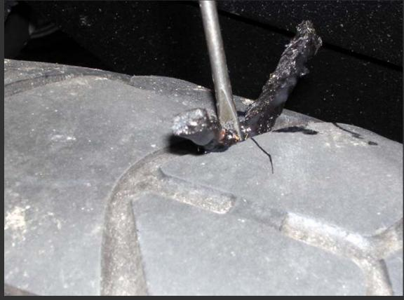
I start pushing in the plug. It is pretty hard to get in, as it should be for a good seal.
