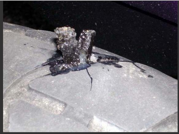
Here is the plug all the way in. Note, make sure you leave at least half an inch. You do this to ensure you don't accidentally push the plug all the way through, and so both sides of the plug remain above the tread.
