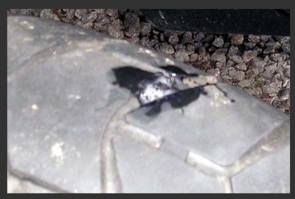
Test the tire for leaks. I used spit, so it looks bubbly, but it isn't, and you can easily see that there are no leaks.
