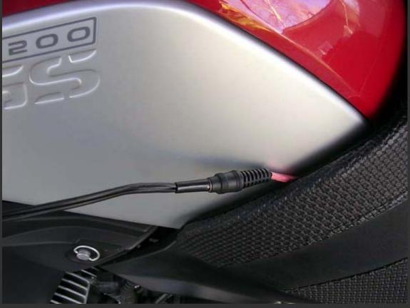
I added a Gerbing style plug to my pump to make it easier to use without removing the seat. I also
