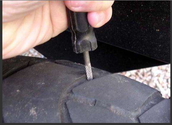
Here is the reamer all the way in. I had to push pretty hard, and I also twist it in the same direction always as I push it in and pull it out, this orients the strands so they are less abrasive to the plug. I gave it 5 strokes.
