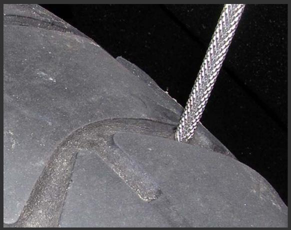
After pulling the nail, I use the reamer tool to make the hole ready for the plug by enlarging it slightly, and roughing up the sides of the hole.
