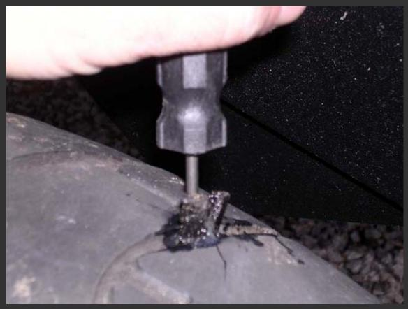
When you get it in this far you stop. Pull the tool straight out as firmly as you can. No twisting. The tool comes out easier than it goes in.
