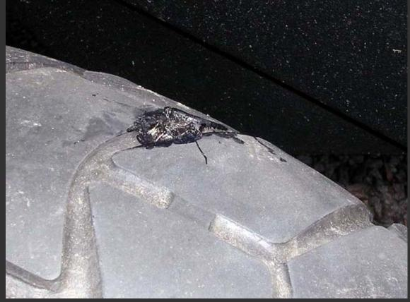
Here is the trimmed down plug. Note that it doesn't have to look good, just be trimmed flush as much as possible.
