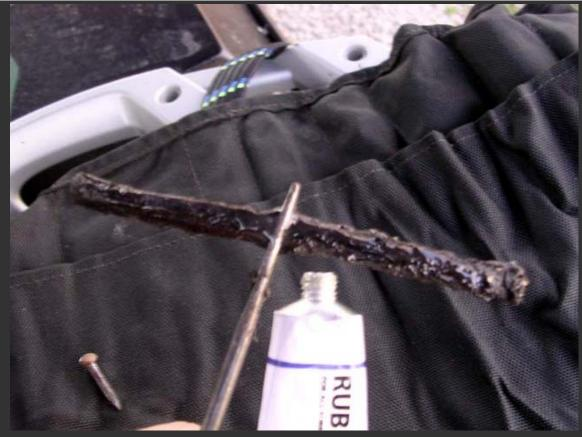
Then I put glue on the string and tool. This not only halps make a more permanent seal, but lubricates it for easier installation.
