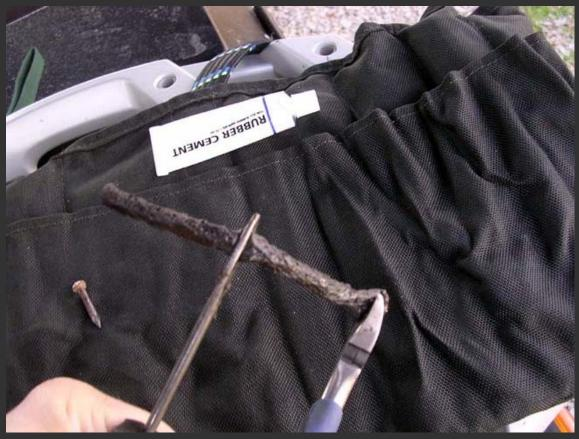
Squish the string plug flat and insert it into the tool. I used the cutters to pull it through since it can be stubborn. There are different types of installer tools, and some have an opening that makes installing the string easier.
